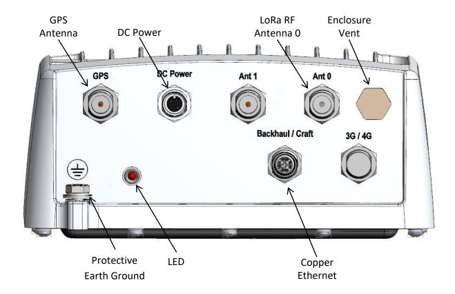
Figure 11: Kona Mega Gateway Option #4 with M12 Connectors Bulkhead Field
