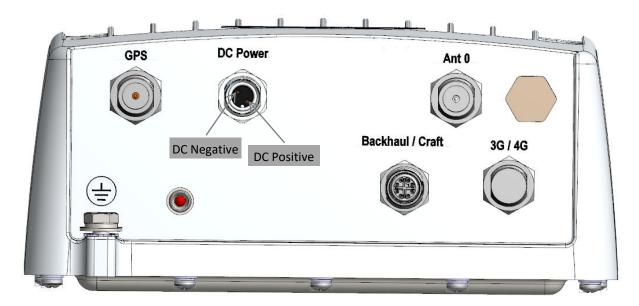
Figure 15: Direct DC Power M12 Connector Connection Polarity
