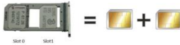
Figure 5: SIM Tray Layout
