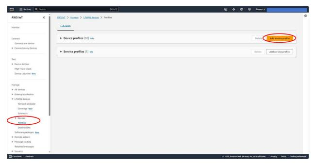
4. Choose "Add device profile" and input your device profile accordingly. Currently CHICKADEE uses LoRaWAN version 1.0.3 and regional parameter v1.0.3rA. Once finished, click on "Add device profile".
