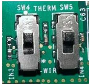
Figure 11: Input 3 and 4 Switches showing “SW4” and “SW5” default positions
