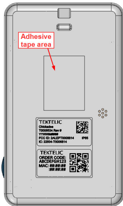
Figure 2-3: Adhesive Tape Mounting Area
