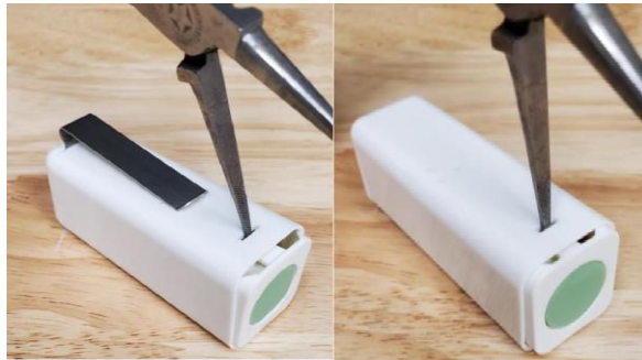
Figure 2-3: Using a Tool to Release the End-Cap
