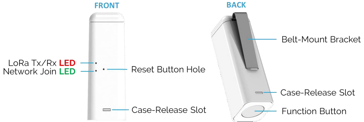
Figure 1-1: FINCH Enclosure and External Interfacing
