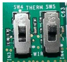
Figure 6: Input 3 and 4 Switches showing “SW4” and “SW5” default positions
