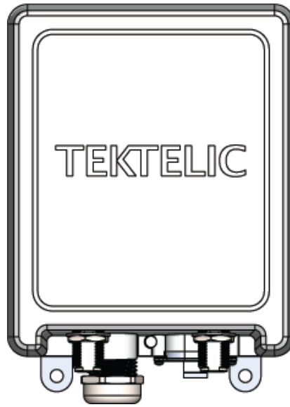
Figure 6: Kona Enterprise Gateway Module Wall Mounting Orientation
