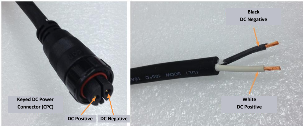
Figure 6: Direct DC Power CPC Connector Connection Polarity
