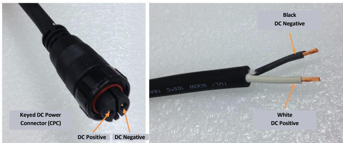
Figure 6: Direct DC Power CPC Connector Connection Polarity
