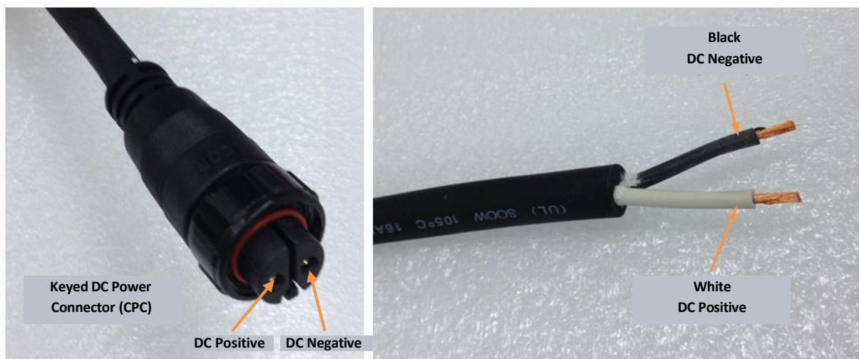
Figure 6: Direct DC Power CPC Connector Connection Polarity
