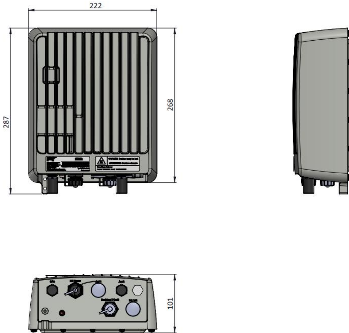
Figure 1: KONA Mega Gateway Common Dimensions
