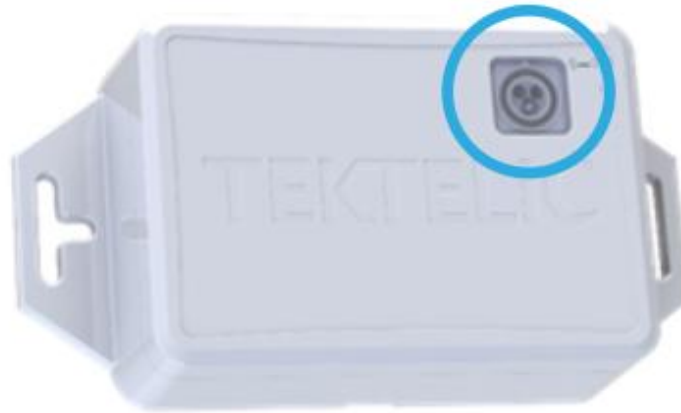
Figure 2-4: The ORCA Enclosure Top View Showing Location of LEDs
