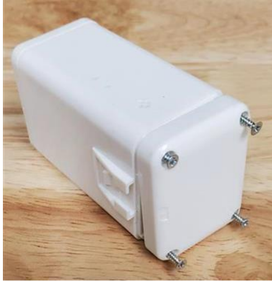
Figure 2-5: Removing the Battery Cover Screws
