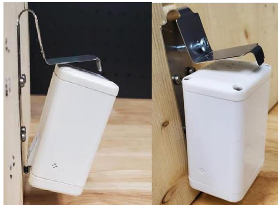
Figure 2-3: Attaching the Tracker to the Mounting Bracket
