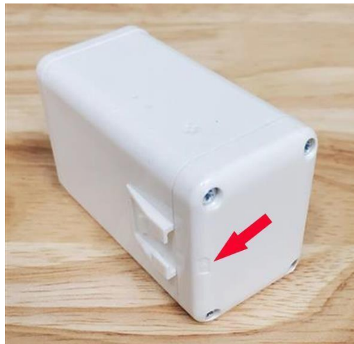
Figure 2-8: Proper Replacement Orientation of the Battery Cover
