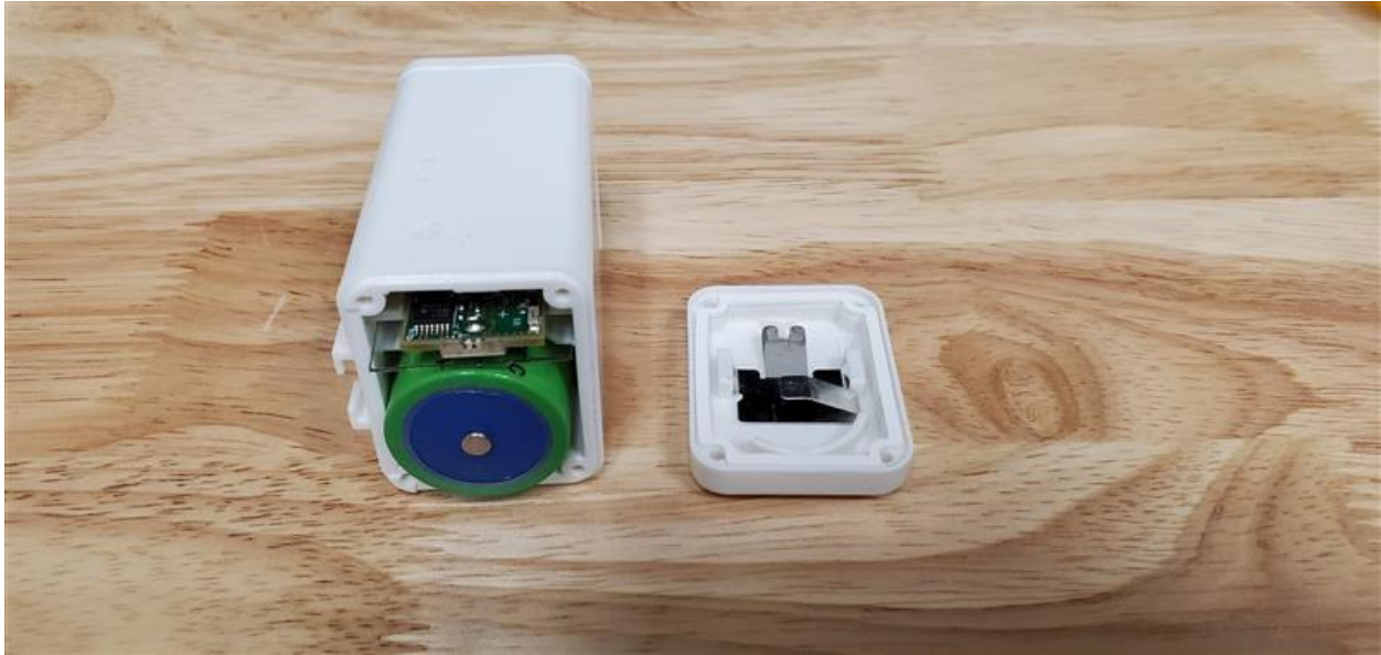
Figure 2-9: Battery Polarity Markers and Insertion
