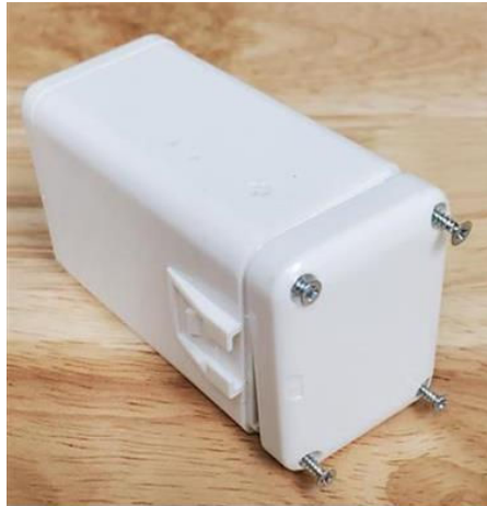
Figure 2-8: Removing the Battery Cover Screws
