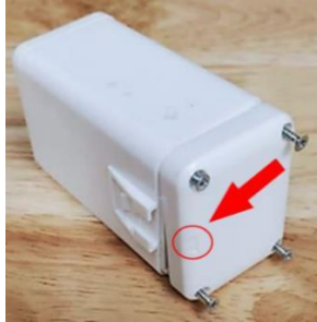
Figure 2-2: Removing the Battery Cover Screw
