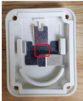
Figure 2-3: Polarity Marker and Battery Insertion
