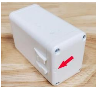
Figure 2-4: Proper Replacement Orientation of the Battery Cover
