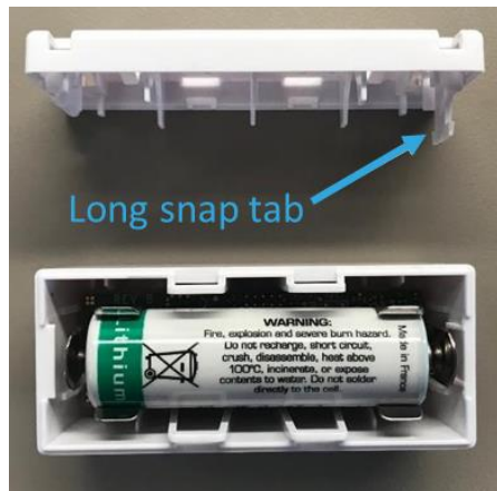
Figure 2-5: Proper Replacement Orientation of the Battery Cover
