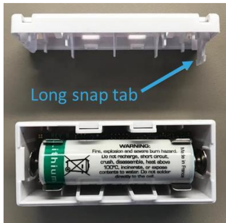
Figure 2-5: Proper Replacement Orientation of the Battery Cover
