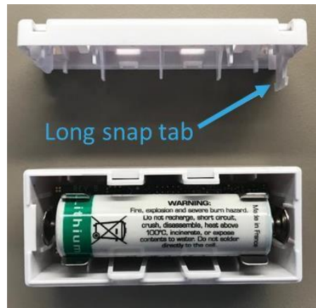
Figure 2-5: Proper Replacement Orientation of the Battery Cover
