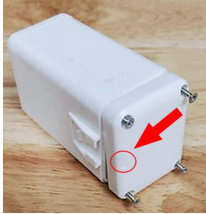
Figure 2-6 Removing the Battery Cover Screws
