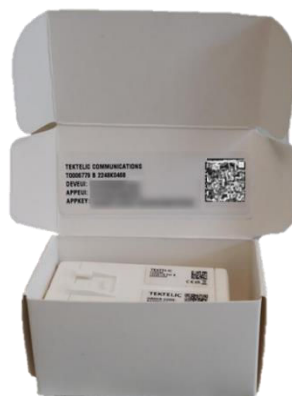
Figure 2-1 TUNDRA Commissioning Keys
