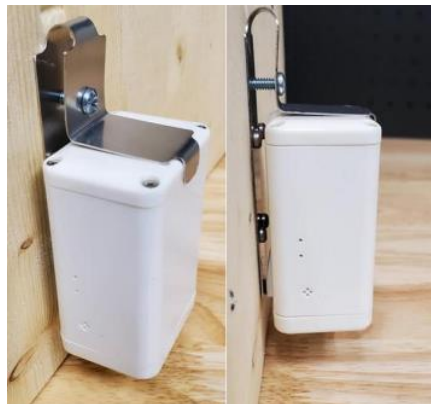
Figure 2-5 Securing the Sensor in the Mounting Bracket with a Fifth Screw
