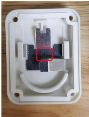
Figure 2-7 Polarity Marker and Battery Insertion
