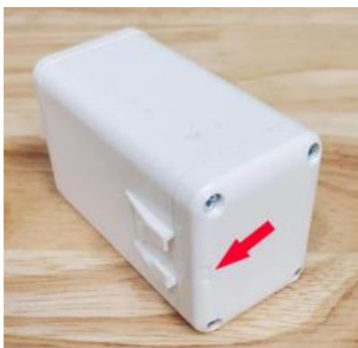
Figure 2-8 Proper Replacement Orientation of the Battery Cover
