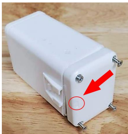
Figure 2-6 Removing the Battery Cover Screws
