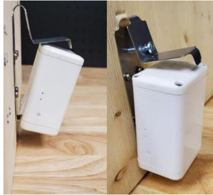
Figure 2-4 Attaching the Sensor to the Mounting Bracket
