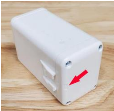
Figure 2-8 Proper Replacement Orientation of the Battery Cover
