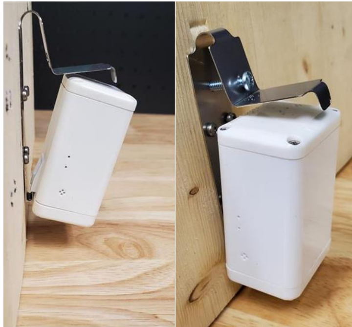
Figure 2-3: Attaching the Sensor to the Mounting Bracket
