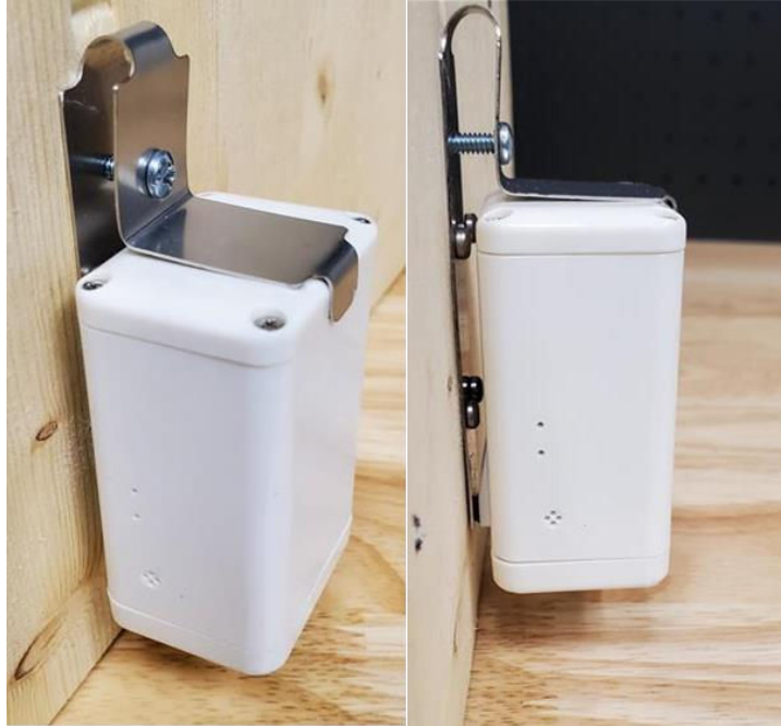
Figure 2-4: Securing the Sensor in the Mounting Bracket with a Fifth Screw
