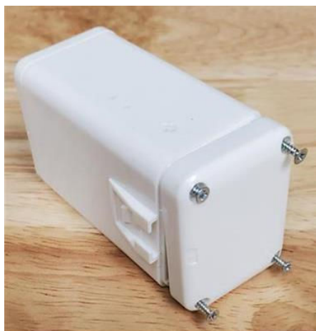
Figure 2-8: Removing the Battery Cover Screws
