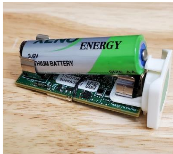
Figure 2-6: Battery Polarity Orientation
